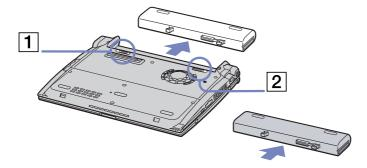
You can remove the battery pack without turning off the computer if it is connected to the mains voltage (AC adapter).
